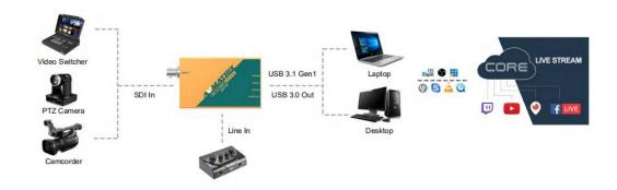
Note: The quality of the broadcast video is guaranteed that the original video is uncompressed and the transmission rate is over 20MB/s. Please make sure to use the interface above USB3.0 rate and the original USB 20MB/s.
