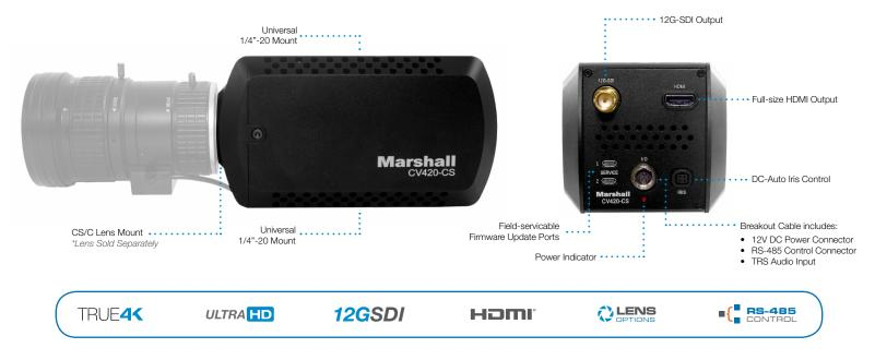
The **Marshall CV420-CS** is a true 4K camera built around a 12.4-Megapixel, 1/1.7-inch sensor delivering ultra-crisp, clear true 4K resolution in 4096x2160p at 60fps. CV420-CS contains a single 12G (BNC) and a simultaneous HDMI 2.0 output covering a variety of 4K/UHD/HD applications. Flexible CS/C lens mount format offers a wide range of lens options with DC Auto-Iris plug-in capability.
