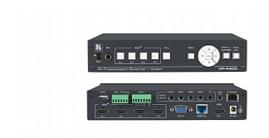
VP-440X is a high-performance 18G 4K HDR presentation switcher/scaler with four HDMI inputs and one computer graphics (VGA) input. It scales the video, embeds the audio, and outputs the signal to two identical outputs – one HDMI and one HDBaseT – together with an analog stereo audio output. Via HDBaseT, it extends video signals to up to 40m (130ft) over CAT copper cables at up to 4K@60Hz (4:2:0) 24bpp video resolution and provides even further reach for lower HD video resolutions
