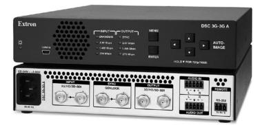
The Extron DSC 3G-3G A is a high performance scaler that converts between 3G-SDI, HD-SDI, and SDI resolutions and frame rates. It accepts SMPTE video resolutions and generates output rates from 480i and 576i to HDTV 1080p/60 and 2K. The DSC 3G-3G A is ideal for applications with professional video systems, including video editing and production, rental and staging, medical imaging, and large-scale presentations.
