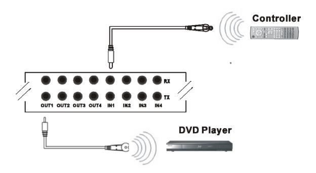
Figure 6-10 IR Extended Aiming – Multimedia
