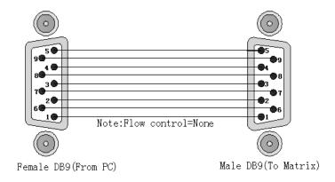
Figure 6-6b RS-232 – From Female DB9 (PC) to Male DB9 (Matrix)
