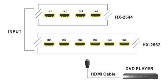
**Figure 6-3 Input Connections**
