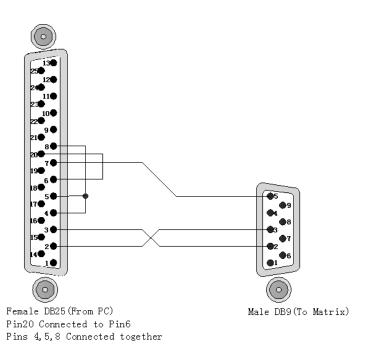
Figure 6-7 RS-232 – From Female DB25 (PC) to Male DB9 (Matrix)
