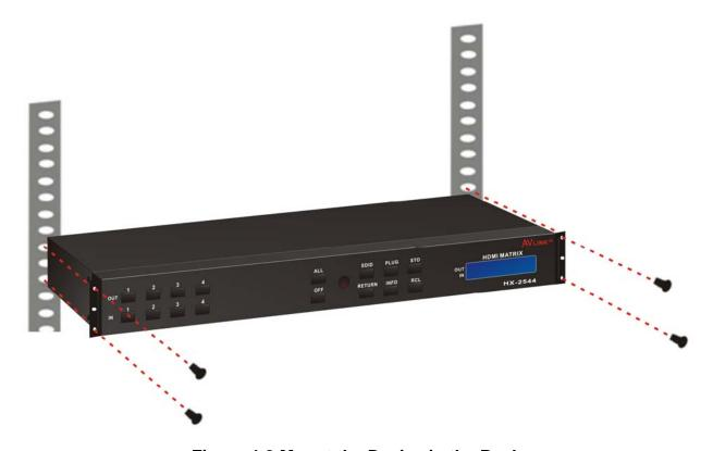
Figure 4-3 Mount the Device in the Rack
