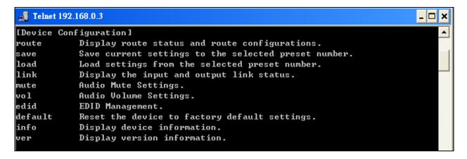
Figure 7-3 Device Configuration
