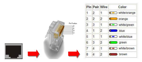
Figure 6-9 RJ45 Connector
