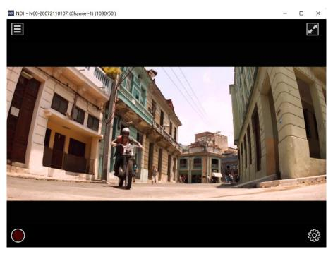
Open vMix, click "Add input" at the bottom left corner, select "more" to display various sources that can be added, click "NDI/Desktop capture" to display the list of NDI sources. Depending on the device name and channel name, you can select the device you want to add and click "OK" to add the selected NDI source to the vMix source list.
