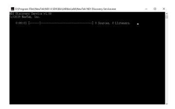
The NDI encoder configures the IP address of the receiving end in the discovery server, and the NDI will be registered to the server. It is recommended that the receiver address be configured as a static IP address to prevent the loss of NDI connections due to IP reassignment.
