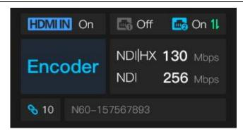
Press the scroll wheel to enter the sub menu, and modify the working mode through choose Model to enter the setting. You can switch from encoding to decoding, and modifying the encoding quality.
