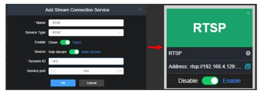
After configuration, it will generate an address, which can be streamed by the backend. This IP address is the address of the current device. Only one RTSP service can be added, while other streams can be up to 5 stream services in total.
