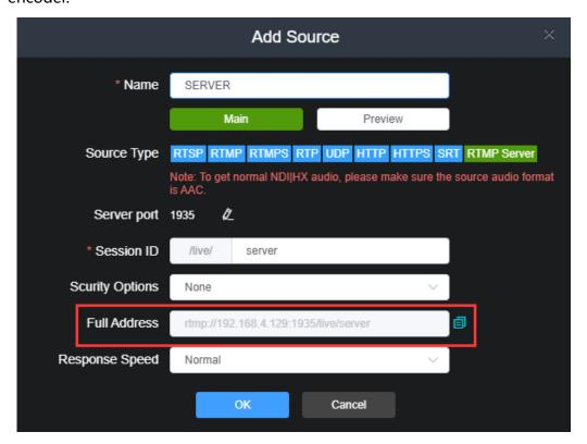
Note: When pushing RTMP from the remote Internet, the U40 needs to have a public network address, and do port forwarding to U40 in the network, and the forwarded port is 1935. The IP address format for RTMP pushing needs to be replaced with a public network address or domain name.
