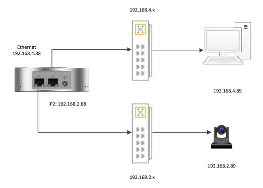
As shown in the above figure, the computer cannot access the camera web page of the other network when the two network ports of the device are connected to different networks. After configuring two IP addresses for U40, your computer can log in to the camera (192.1618.2.89) web page through the Camera link function in Web page of U40.
