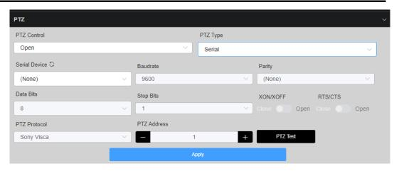
Application 1: PTZ camera supports serial port control. Connect the U40 device through the USB to RS232/RS422/RS485 adapter (cable), and receive the PTZ command converted from the device for control. Both Kiloview NDI decoder and other NDI-enabled PTZ software can be the receiver.
