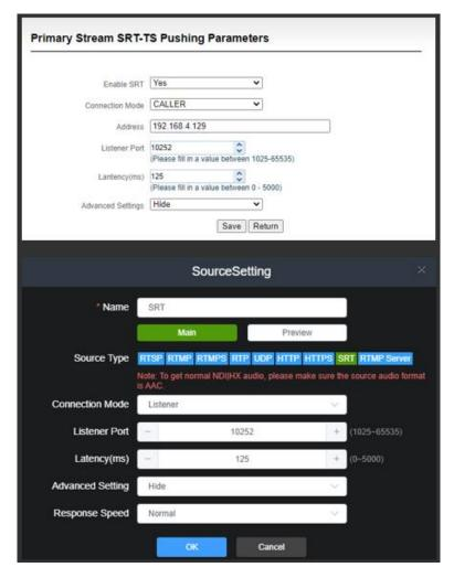
Note: When pushing SRT from the remote Internet, either end of the encoder or U40 needs to have a public network address, and use UDP for port forwarding in a network router with a public network address. The forwarding port range is 1025-65535. For devices without a public network address, please adopt the CALLER mode, fill in the other party's public IP address and port number. The device with public network uses Listener mode, and the port is same as the device setting with CALLER mode.
