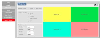
• Window Source: To change the source for a specific window, click on the dropdown next to the window to change (1~4) and select the preferred Input. The switch will occur immediately.
