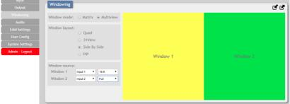
Window Source: To change the source for a specific window, click . on the dropdown next to the window to change (1~2) and select the preferred Input. To change the aspect ratio of the source, as displayed within the window, click on the second dropdown and select "Full", "16:9", or "4:3". The switch or format change will occur immediately.
