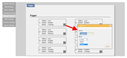
Click on the "Trigger Settings" tab to view the current trigger status and edit trigger behavior. Each trigger has 3 indicators: Status, Active, and Mode.
