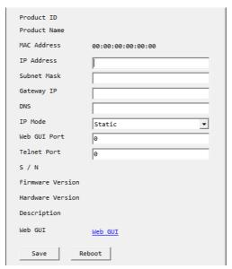
Then user may use the IP Address to find the control device through Telnet, WebGUI or even RS-232/Hyper Terminal tools.
