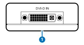
**1 DVI-D IN:** Connect to the DVI equipped source equipment such as a PC or notebook for DVI input signal with a DVI cable.
