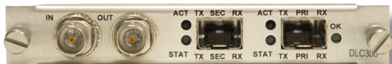
Rear panel Includes electrical input or output and dual SFP transceiver cages
