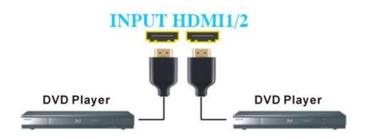
Figure 6-2: Input Connection-HDMI
