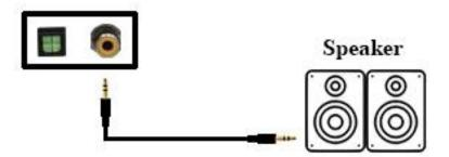
**Figure 6-5: Audio Output Connection**
