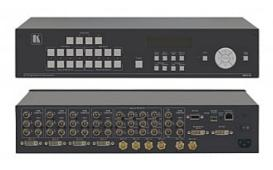
The MV-5 is a versatile, high-performance video and graphic multi-window viewer for DVI signals, SD and HD analog signals up to 1920x1200@60Hz, and SDI signals up to 3G HD-SDI. The device can window up to four sources (plus a background) in any layout and output the image as SDI, DVI, component and composite video signals. Both preprogrammed and customizable screen division is supported
