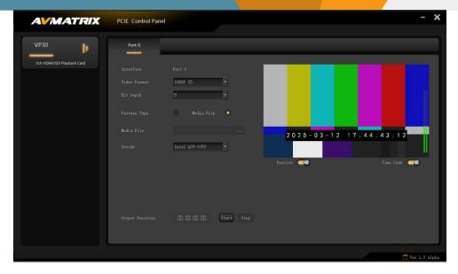
After the user has completed the settings, click "Start" to output. Preview and timecode can be turned on or off according to the user's needs.
