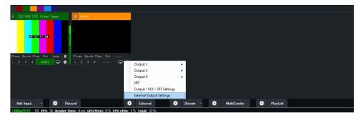
Step 2: Select "VP30" as the video output device in the external output settings.
