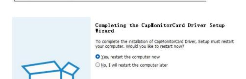
In particular, if any of Blackmagic Design's PCIe capture or output card drivers are already installed on computer, pls uninstall it before installing the AVMATRIX PCIe card driver. Otherwise, the AVMATRIX PCIe card will not work properly.
