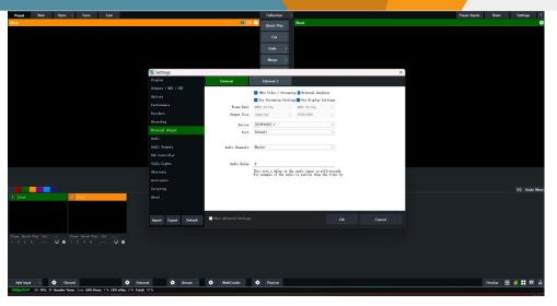
Step 3: When the setting is finished, click "External", the icon will turn red, and the output will start.
