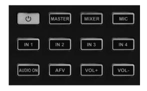
When the indicator of button in Part A is on in green means the corresponding audio is on. When the indicator is off means the corresponding audio is off.
