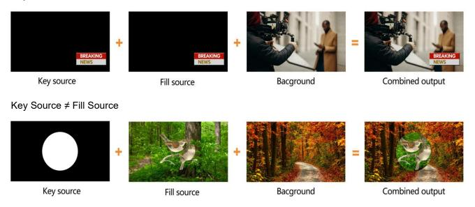
Luma key provides a way to composite a Text clip over a background clip based on the luminance levels in the video. Turn on the Luma Key, a color from the key source will be removed, revealing another background image behind it.
