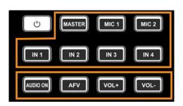
Part A is for selecting one audio to be configured, including Master, MIC 1, MIC 2, IN 1, IN 2, IN 3 and IN 4.
